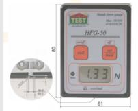
For mounting to the holding support (test stand), use 2pcs. M4 screws, Min.length of screws = support thickness + 7mm, Max. length of screws=support thickness+11mm, no longer!
